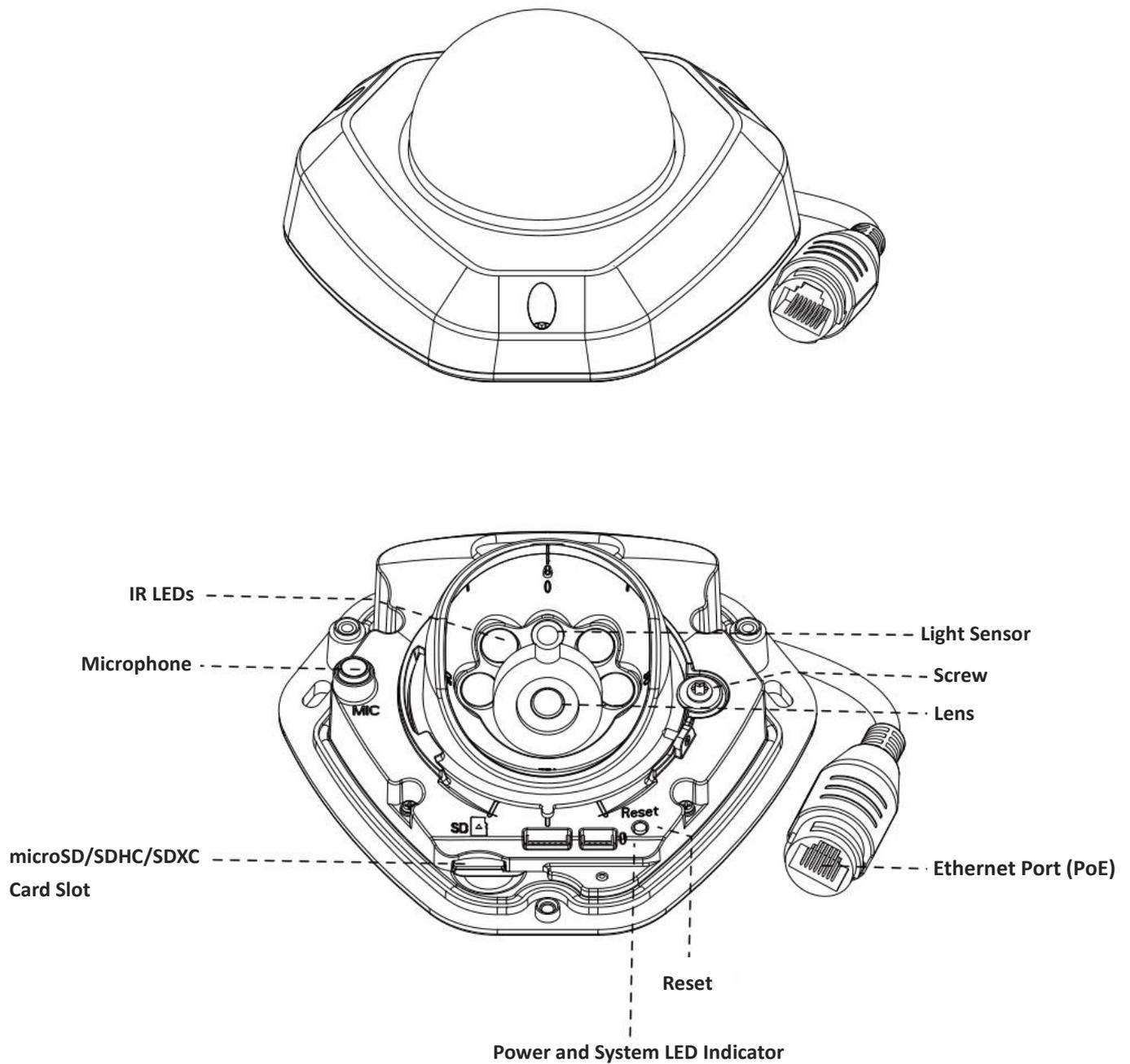
Figure 1-3-3 Vandal-proof Mini Dome Network Camera
