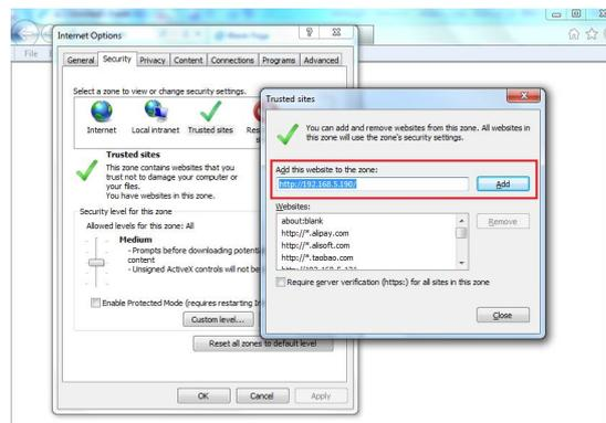
Step4: Enter the IP address. After logging on network camera's web GUI successfully, user is allowed to view live video as follows.
