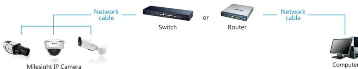
Figure 2-1-2 Connect via a switch or a Router
