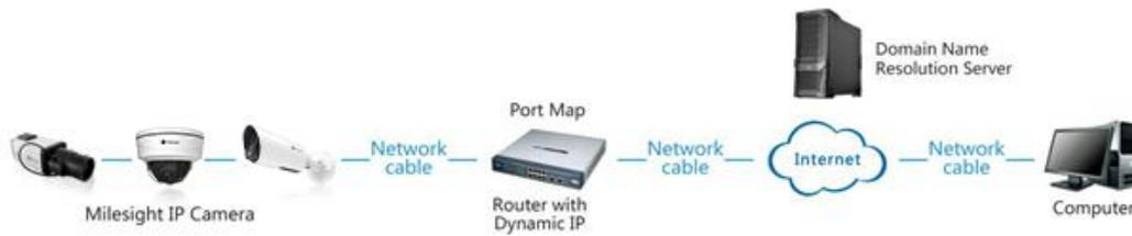
Figure 2-2 Connect the network camera via a router using dynamic IP
