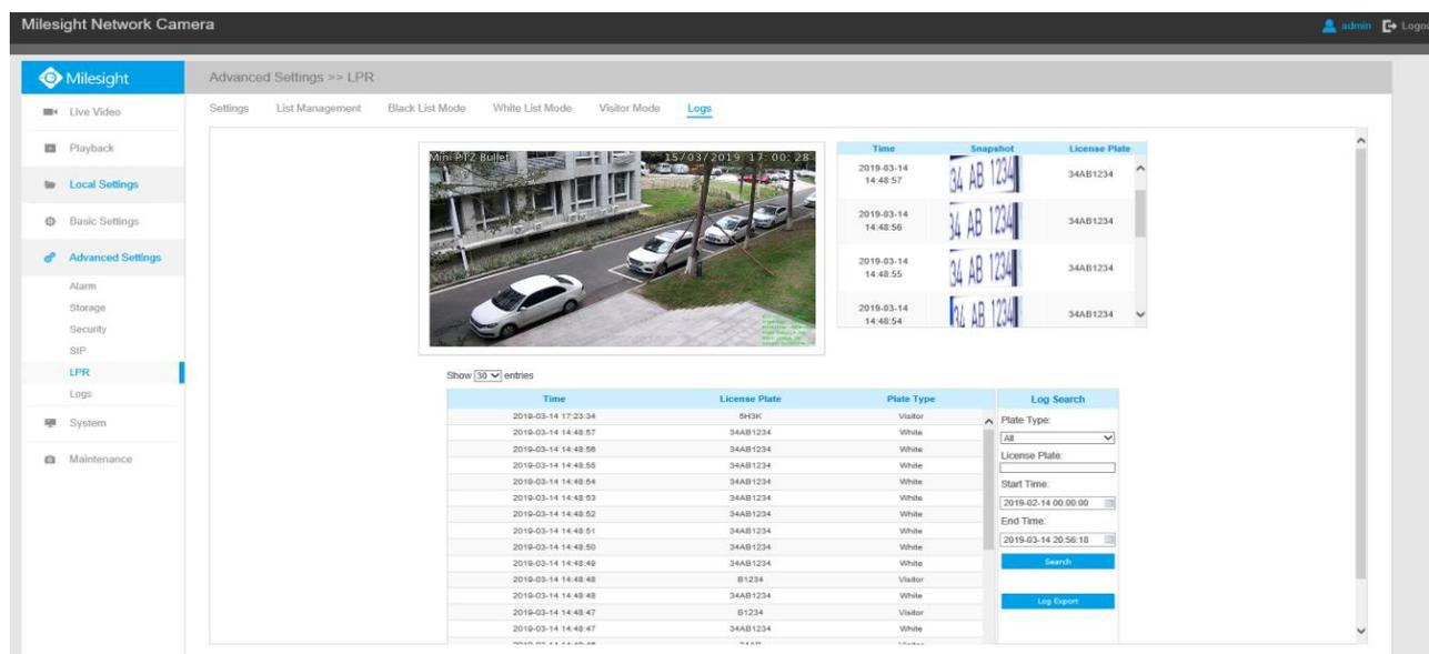
The detect results in real time will be displayed on the right side of Logs page, including detected time, live screenshot, and license plate.
