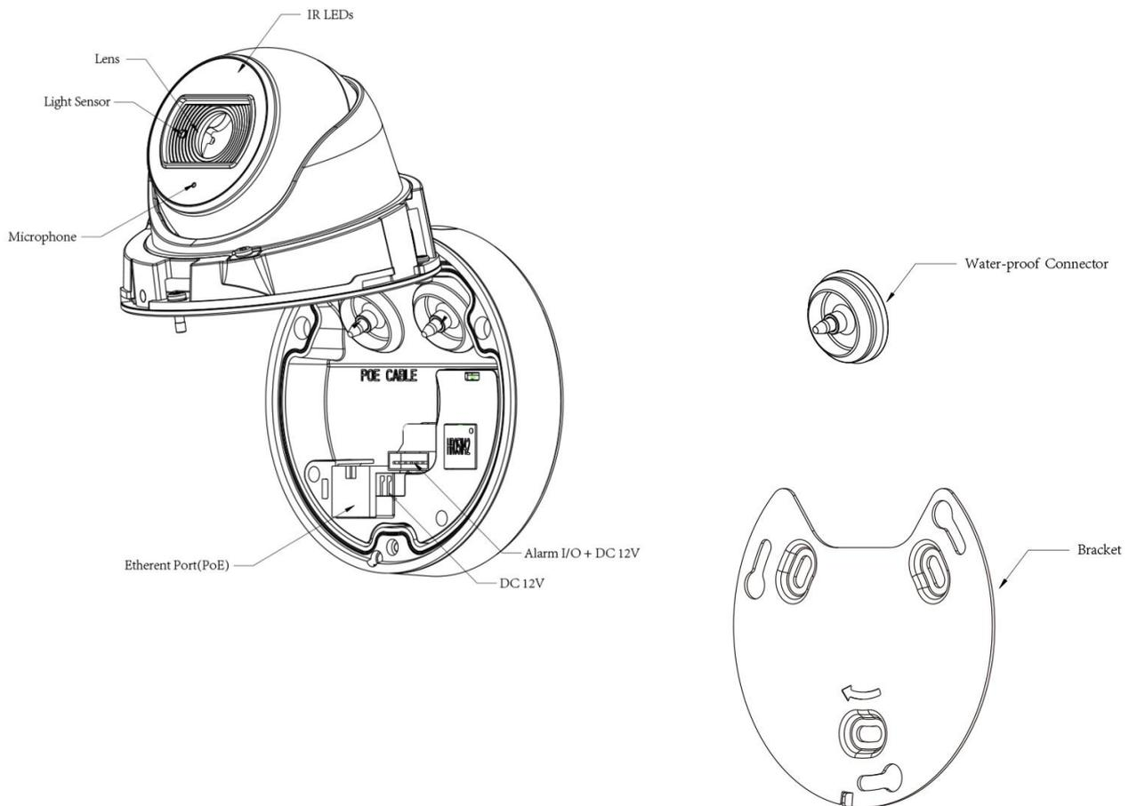
Figure 1-3-5 AF Motorized Mini Dome Network Camera
