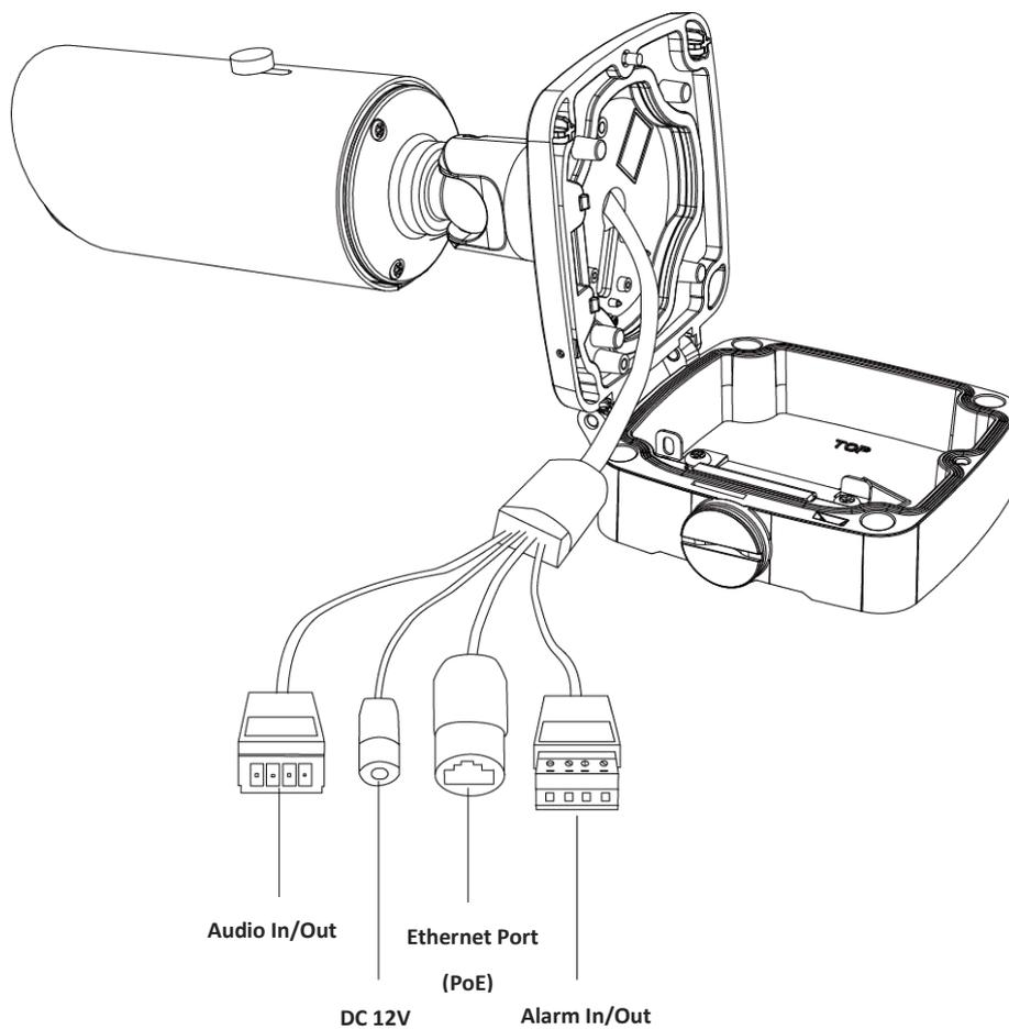
Figure 1-3-11 Motorized Pro Bullet Network Camera (Version B)
