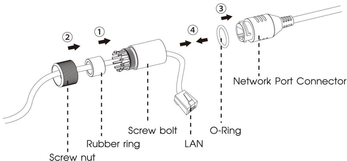
Step1: Get the network cable through the screw nut, rubber ring and the screw bolt.
