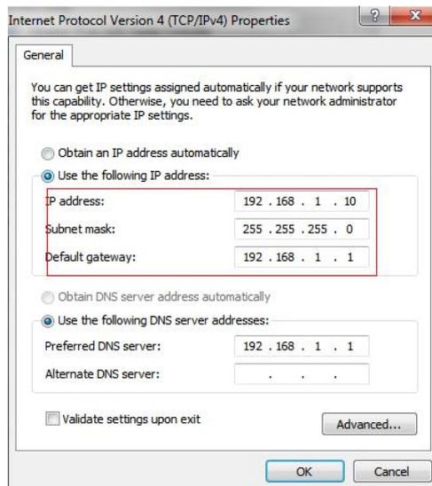
Figure 3-1-8 Setting Network Segment IP Address of Computer
