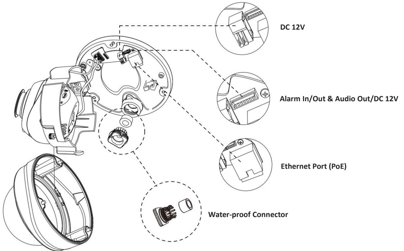
Figure 1-3-13 Motorized Pro Dome Network Camera multiple interface
