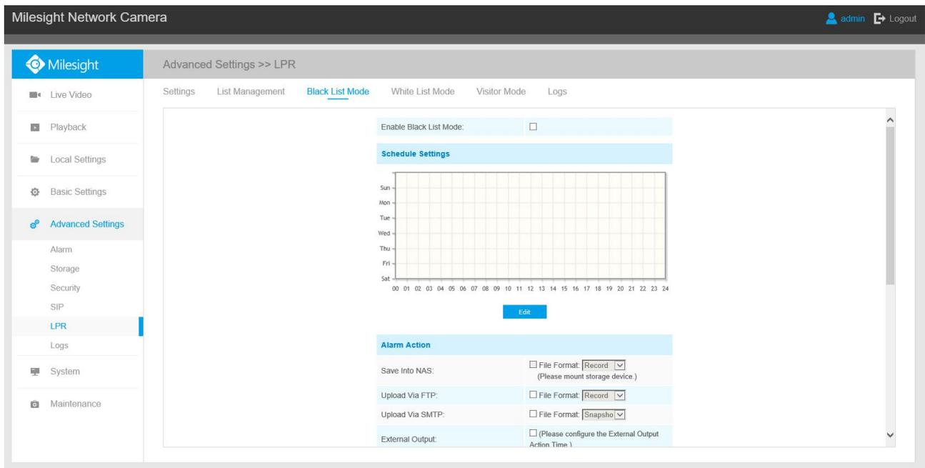
Step1: Check the checkbox to enable Black List Mode.
