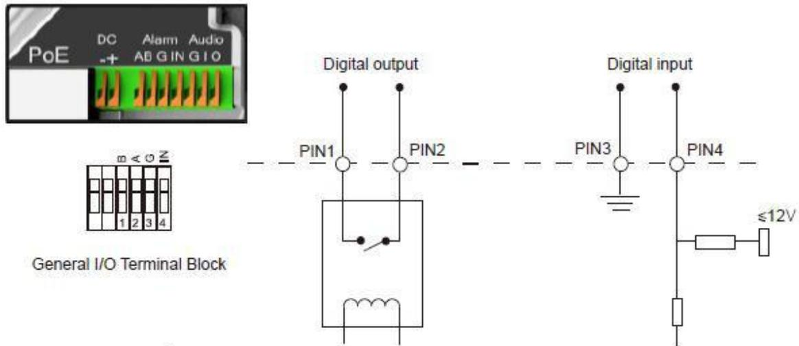
PIN1: Alarm Output NC/NO 24V DC 1A
