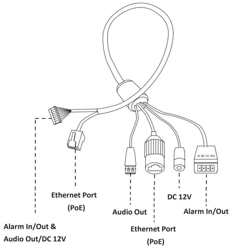
Figure 1-3-14 Motorized Pro Dome Network Camera multiple interface cable
