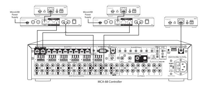
Make sure to adjust the "Source Number" rotary dial on the bottom of each BTC-2X to correspond with the source number being used for the audio input on the Russound controller and to configure the same audio source in the controller's Web Config as a "BTC-2X".
